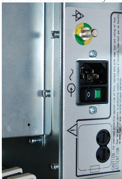
Fig. 3-3: Main switch on the rear of the device
